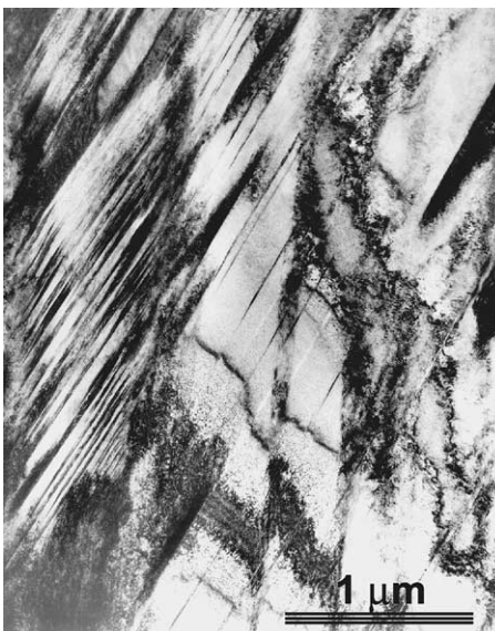
Fig. 5. Micrographs showing the twin structure in deformed 316L steel containing 0.5 at.% He.
